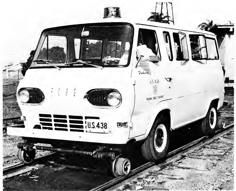
A "whachamacallit?" No, there really is a name for it—the "rail-car" in railroad language. Two of them have been purchased for the Railroad Division and are used for track patrol and inspection. They can carry seven passengers and a driver and could be used to supplement train schedules. The small steel wheels substitute for rubber tires.
